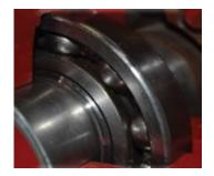
down. For easy maintenance, Kinamatic motors have antifriction bearings and removable bearing cartridges and caps.
