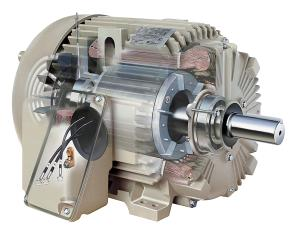
Rotor assembly balanced to ISO 1940 Grade 1.0 for low vibration. The vibration level is 50% lower than the requirement of IEEE 841-2009 Standard and can increase bearing life by as much as 60%.
